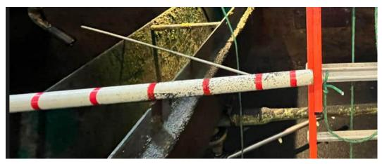
Figure 4. Backwash Bed Expansion Tool
