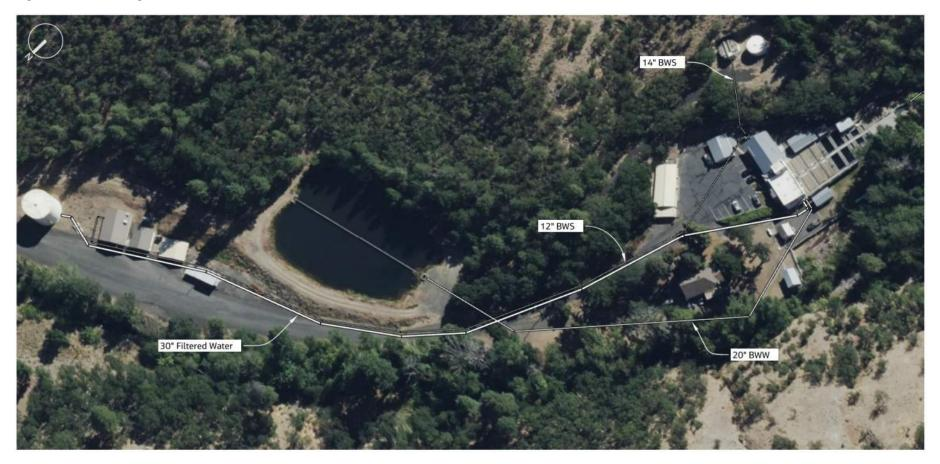
Figure 10. Phase 1A of Wicks WTP Construction
