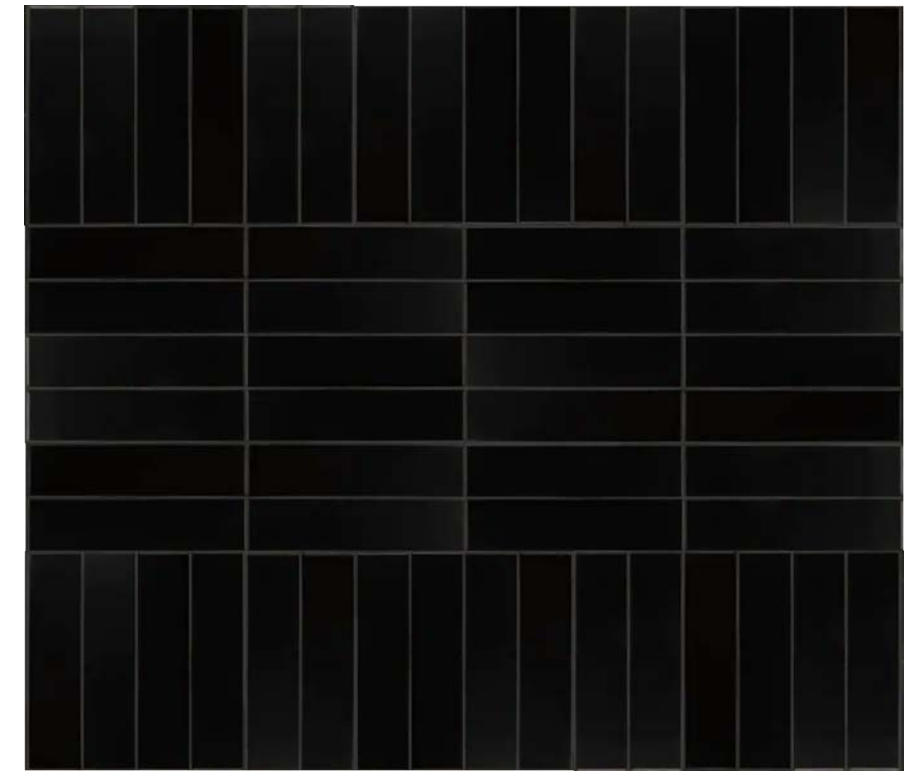
subway tile layout, horizontal stack with vertical boarder at top & bottom
