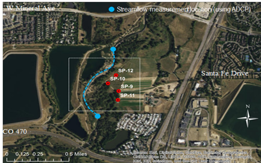
Figure 1. Map of study area, showing location of 4 pumping wells and the location of streamflow measurements.
