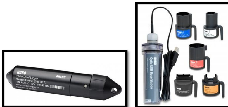
Figure 6. Left : HOBO Water level data logger (Part #U20L-01) Right : Optic USB Base Station to connect the data logger to a laptop for downloading water level data.
