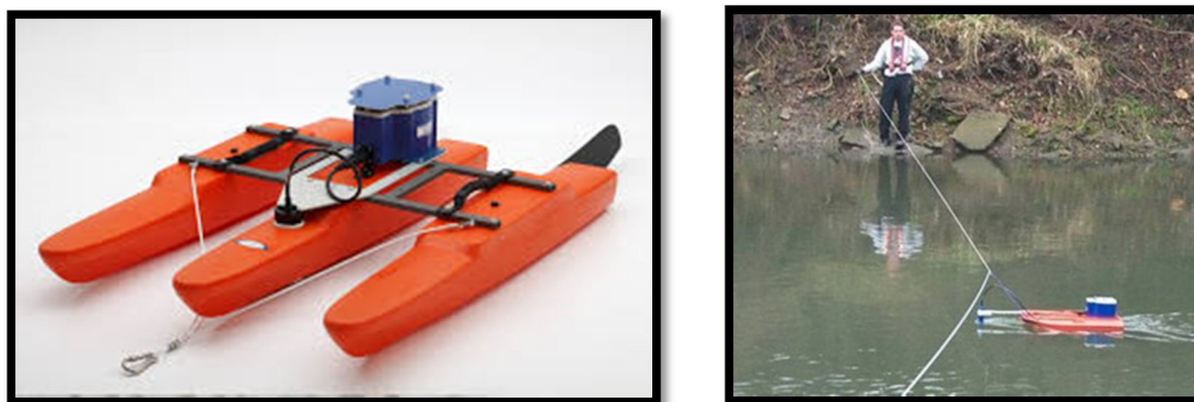
Figure 2. Acoustic Doppler Current Profiler used to measure streamflow in a river.
