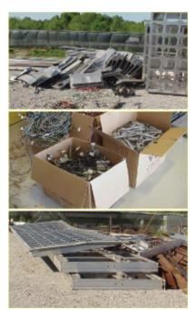
Aluminum comprises more than 64 percent of an LED billboard, which also yields stainless steel and copper wire and LED modules with metal content.
