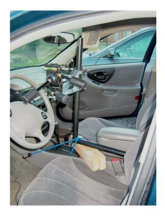
Figure 34. Bracket for Radiant Imaging CCD Photometer.
