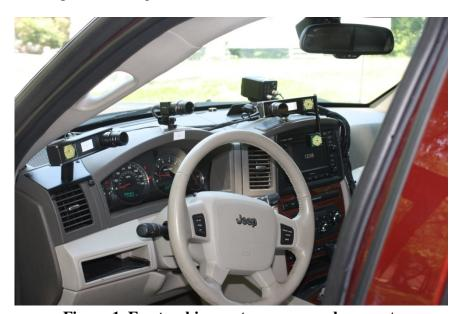
Figure 1. Eye tracking system camera placement.
