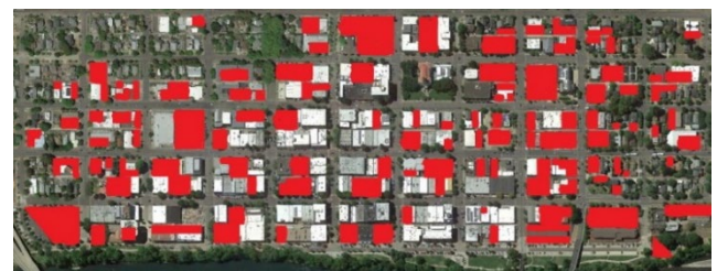
Parking uses a huge amount of high-value land. Off-street parking in downtown Corvallis in red.
